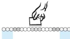
Apply the product on the screen with a brush and leave it in action for at least 1 hour. (the frames may also be left up to 12 hours)
