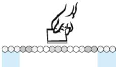
After the recovery operation with **POLISTRIP** and detected the presence of traces of emulsion residues (mainly at the crossing areas of the mesh of the fabric) apply **SOLVENT 610** through the use of a brush. Rub the surface to facilitate the penetration of the product. Leave for 5-10 minutes
